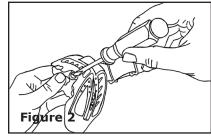
**WARNING:** The right and left gray retention clips are not the same. The back of each clip is marked either "L" for left, or "R" for right. Make sure that the Dye logo on the strap faces up. When properly installed the top of the strap attachment clip is flush with the goggle.
