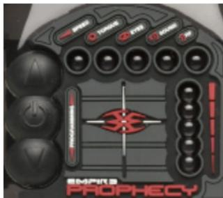
**Cycling through Functions-** Once you have entered Programming Mode, use the Power
