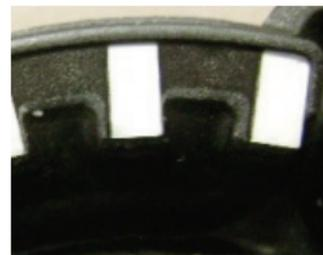
**Sprocket Encoder Decal-** Included with the LTD kit is a new sprocket. The LTD sprocket will have the encoder decal already attached. Simply replace the original sprocket with the new LTD sprocket.
